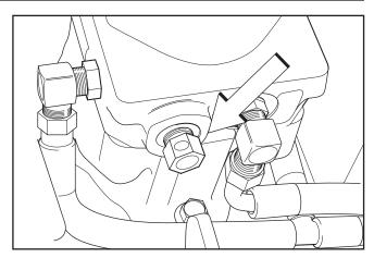
Vent screws on the hydraulic pump
